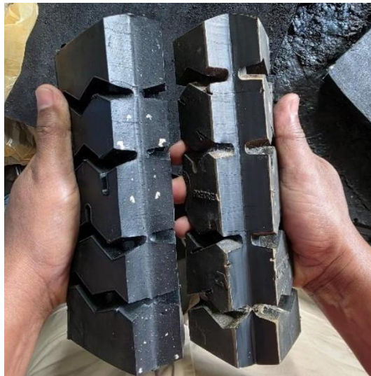
Figure 20: Tread liner with visible contamination affecting quality
