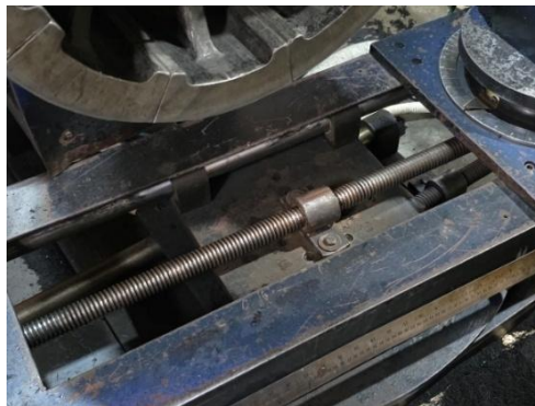
Figure 10: Centre of the tyre and centre of the cutting bed are not aligned
