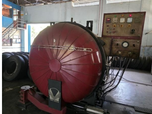
Figure 13: 11 Tyre Electric curing chamber
