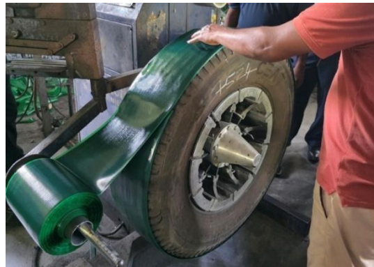
Figure 17: Excess width of cushion gum causing gaps and difficulty in inspection.
