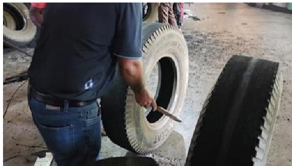
Figure 26: Checking worn out tires using a metal piece
